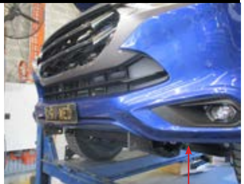
Black plastic lower bumper trim removed
