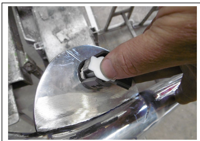
Figure 7: Insert sensor into housing. Type 8 shown
