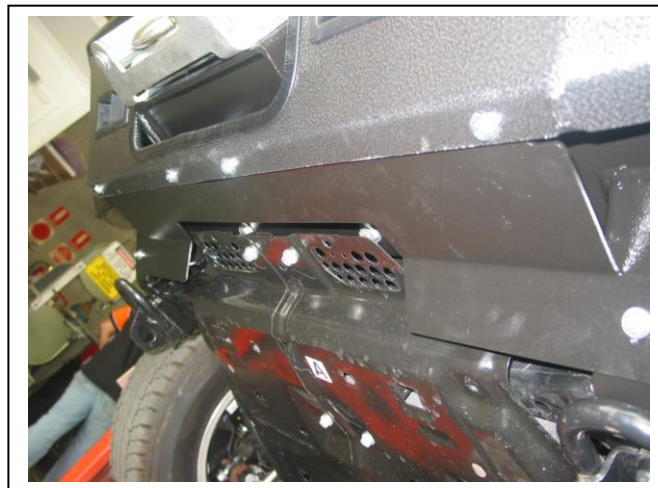
Figure 17: Centre under body guard fitted.
