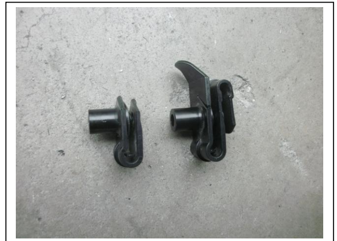
Figure 12: Cut down lower bumper clips for use on rear of inner guard
