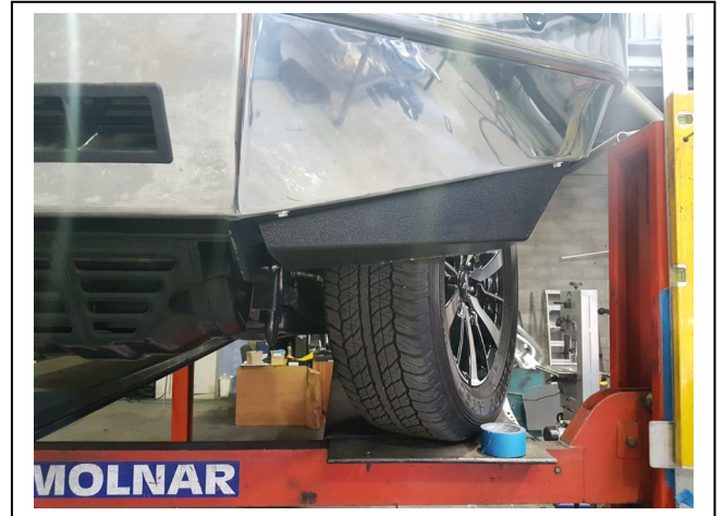
Figure 16: liner trimmed to fit guard
