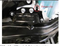
Fit to tow pin hole in vehicle cross member using M10 x 1.5 x 120mm bolt, flat washer, spring
