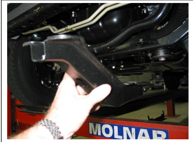
Figure 9 – Shown removing cross member supports
