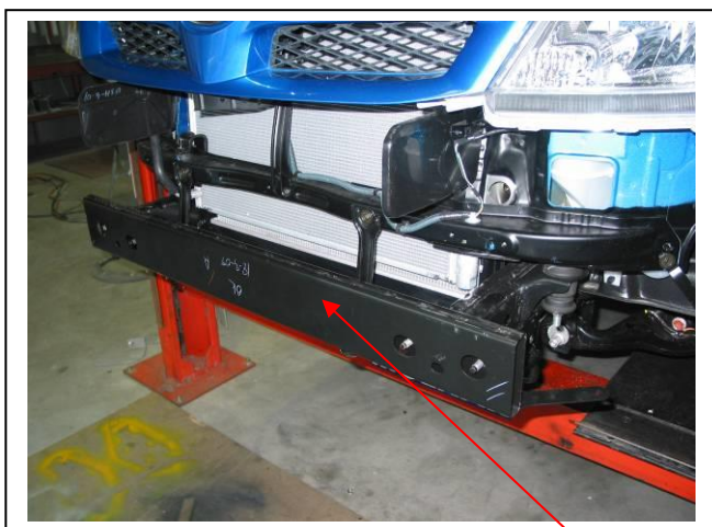
Figure 1 Remove original cross member
