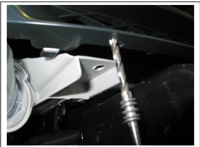
Figure 7 – Drivers side Shown. Shown drilling lower lip of grille
