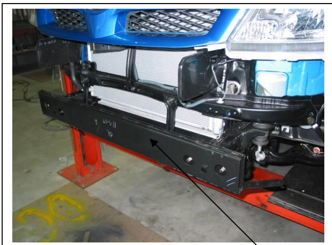
Figure 1 Remove original cross member
