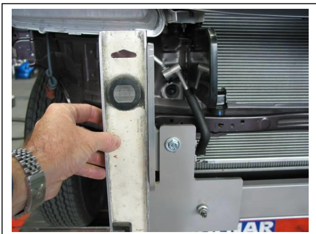
Figure 15 – Drivers side shown Levelling at sides
