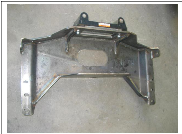
Figure 3 – Drivers side shown Drill two 13mm holes top of chassis, Drivers and passengers side
