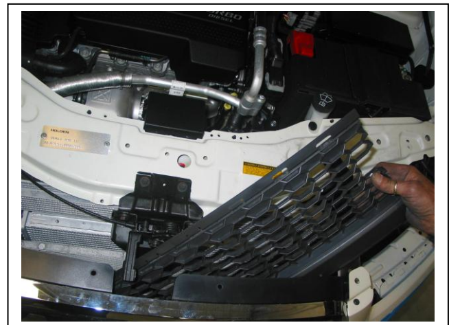
Figure 12: Slide trimmed grille behind bumper and clip into place.
