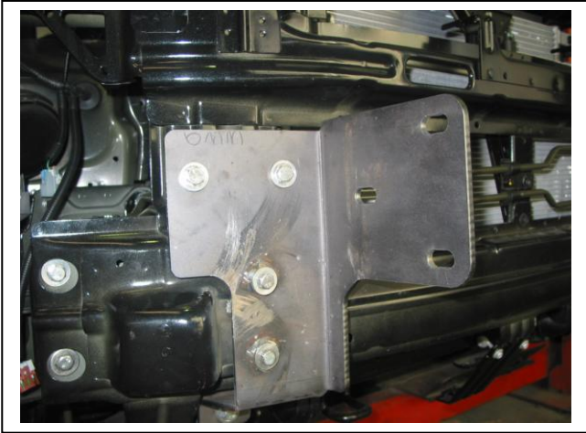
Figure 3: Outer mounting bracket fitted to front of radiator support
