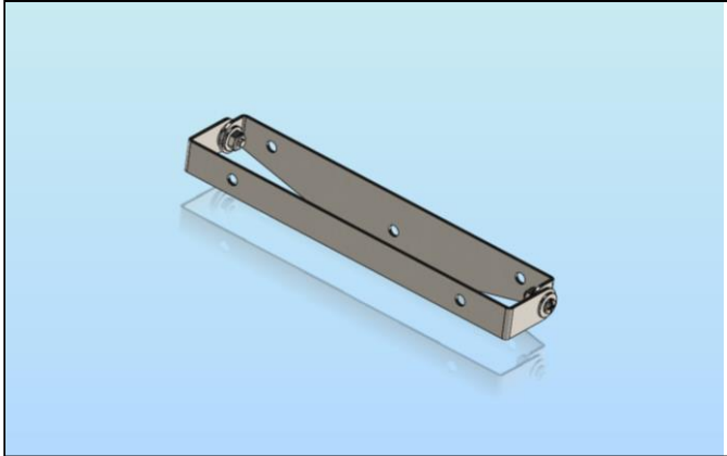
Number Plate mount assembly Number plate hinge plate A Number plate hinge C 40_A3Al
