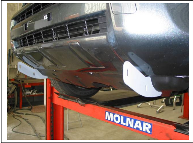
Figure 5 – Plastic under guard shown refitted around steel mounting brackets.
