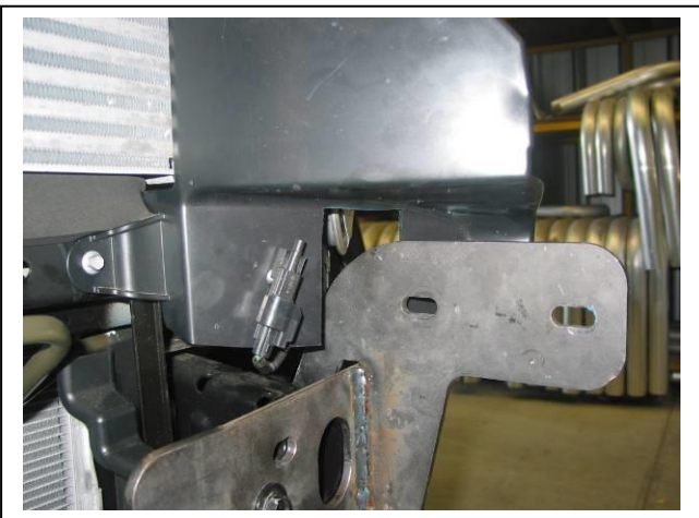
Figure 8: Drivers side air dam trim. Note: Air temp sensor refitted behind cut out.
