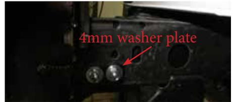
NOTE: 4 mm packer plate (supplied) may be needed between rail and mount, as some chassis rails may vary from side to side. Ensure mount is central to body.
